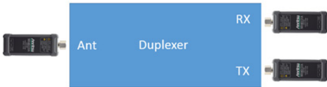
Figure 3-8. MS46121As Setup Up to Measure a 3 Port Device
